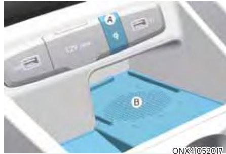
[A] : Indicator light, [B] : Charging pad
